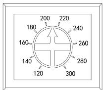
**Note:** To protect the motor, set the arrow number as the same as the motor nominated power. Whenever overload occurs the drive will turn out to be the protection mode.
